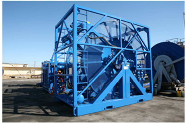
Figure 8. Coiled tubing reel, 22,000 ft. to 2 inches [13].
